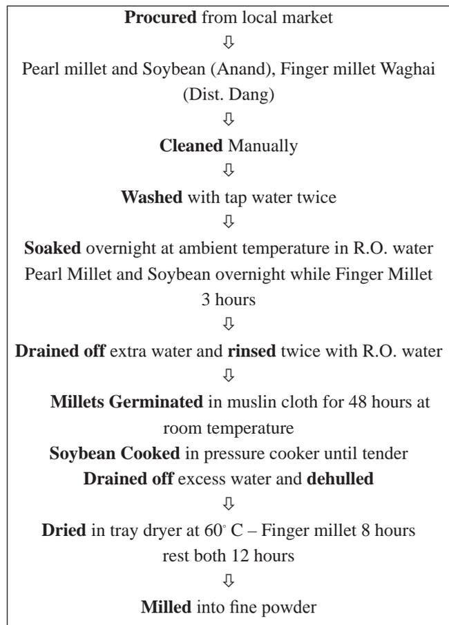
Figure 1 : Flow chart for grin processing
